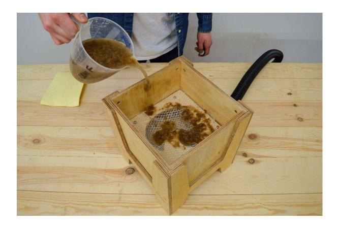
Connect the wet and dry vacuum to the pipe on the bottom of the FORMiT tool and turn it on. Start to gently pour the paper pulp over the mould and make sure to evenly cover all of it. As you cover the mould the pressure under will increase and change the sound of the vacuum, which is nothing to worry about!
