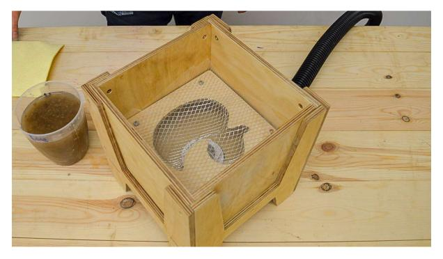
Place the mould inside the FORMiT tool and add the nylon mesh square over the top. This mesh is for collecting the paper fibres onto and helps the pieces to keep their structure while they dry.
