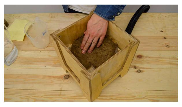
Once of all the mould is covered leave the vacuum running for a minute or so. Use your hands to push the paper against the mould and even out the internal finish. The suction will pull most of the water out of the pulp and you should see the pulp become lighter in colour. Now turn the vacuum off.
